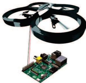
Figure 3: An image depicting the AR Drone hardwired to a Raspberry Pi GPIO pins
