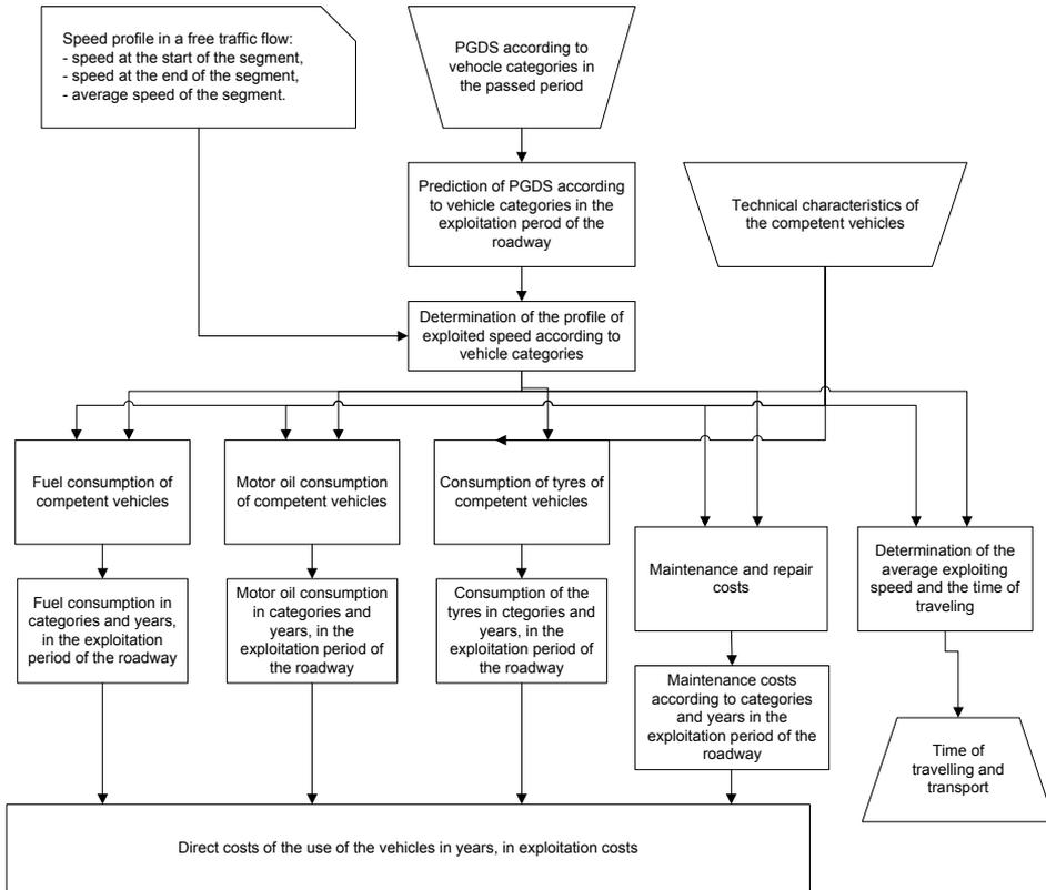
Figure 3: Block diagram of the module for determination of the direct exploitation costs of the roadway
