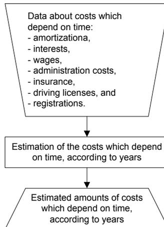
Figure 4: A block diagram of the module for determination of costs that depend on time
