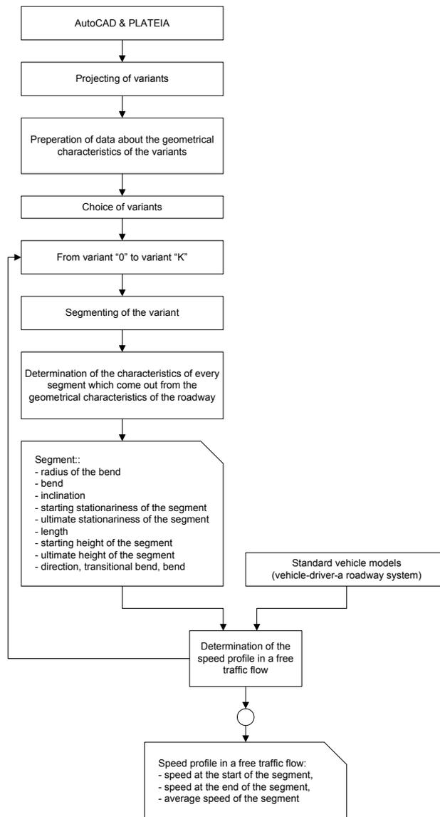
Figure 2: Block diagram of the module for determination the speed of free traffic flow
