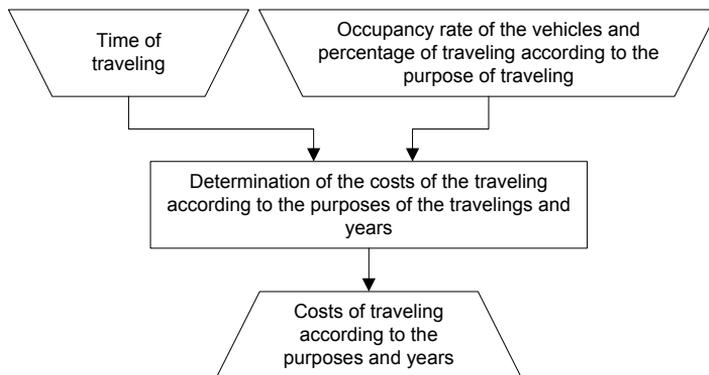
Figure 7: A block diagram of the module for determination of the costs for the time of traveling of the passengers.
