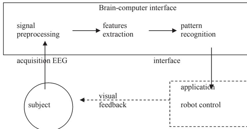
**Fig. 4.** Block diagram of a brain-computer interface
