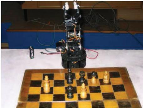
Figure 3: Chess playing using the robot arm Lynx 5
