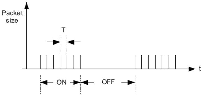
Figure 1: Characteristics of a VoIP single source.
