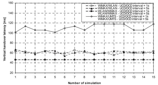
Figure 3: Vertical handover latency between WiMAX/WLAN, WLAN/WiMAX and WiMAX/UMTS networks for VoIP (G.723.1) traffic for 15 simulations of random mobile terminal trajectories.
