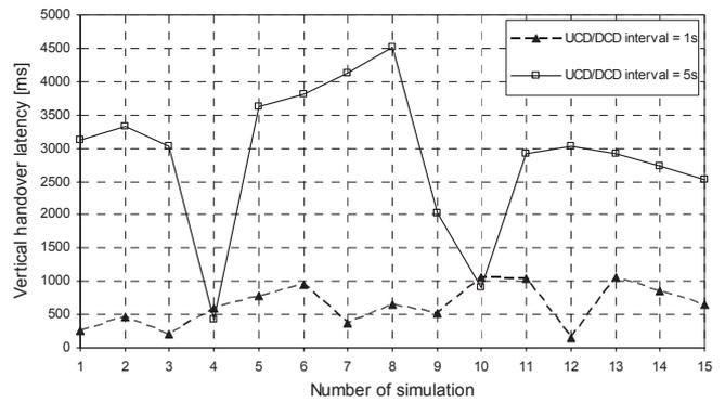
Figure 2: Effect of varying DCD and UCD interval on vertical handover latency between UMTS and WiMAX networks for VoIP (G.723.1) traffic for 15 simulations of random mobile terminal trajectories.
