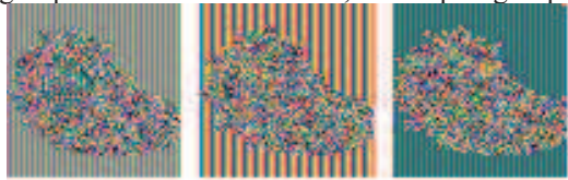
Figure 8: Encryption of (1) with the quasigroup number 576. This shows that the CBC mode is far more convenient for the use of encrypting images with SQBC than the ECB mode. Also, the original image (1) was encrypted using 8 bit block and ECB mode, with the original concept of the SQBC algorithm [1] where the first block is encrypted with one and all other blocks with another algorithm. The quasigroups used were quasigroup number 1, quasigroup number 6 and quasigroup number 181. Figure 9 shows the results.
